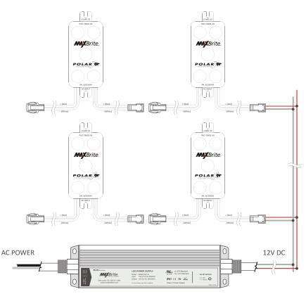
Maximum driver quantity per serial connection is limited. Using more quantity per run will cause overload from Power Supply which damages all connected products. This will cause voltage drop and dimmed lighting output.
